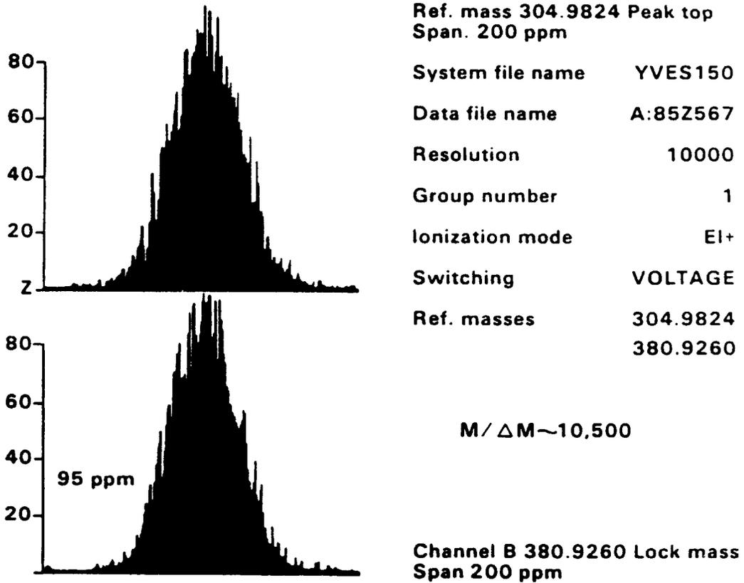
Peak profiles representing two PFK reference ions at  $m/z$  305 and 381. The resolution of the high-mass signal is 95 ppm at 5 percent of the peak height; this corresponds to a resolving power  $M/\Delta M$  of 10,500 (10 percent valley definition).
