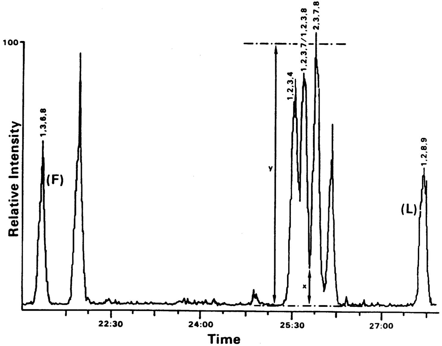
Selected ion current profile for m/z 322 (TCDDs) produced by MS analysis of the GC performance check solution on a 60 m DB-5 fused-silica capillary column under the conditions listed in Sec. 7.6.
