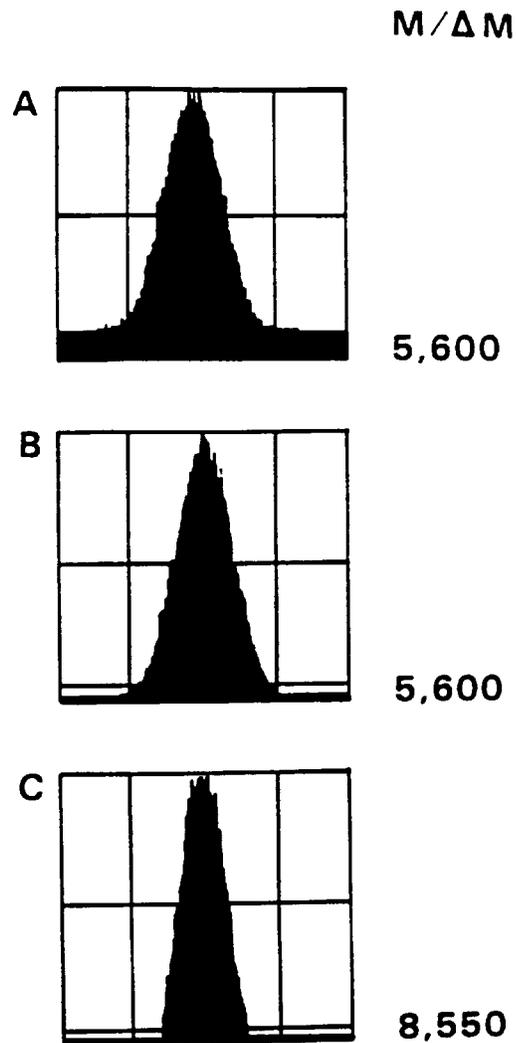
Peak profile displays demonstrating the effect of the detector zero on the measured resolving power.
